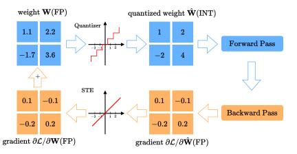
Schematic view of a QAT procedure with STE applied (adapted from  $[GKD^{+21}]$ )
